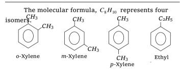
These are produced along with benzene, toluene and ethylbenzene when aromatisation of  $C_6 - C_8$ fraction of petroleum naphtha is done. The xylenes are isolated from the resulting mixture (BTX) by fractional distillation.
